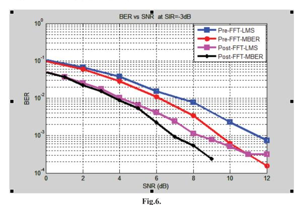
Bit error rate performance (6 antenna elements, 3 users, SIR=-3dB)
