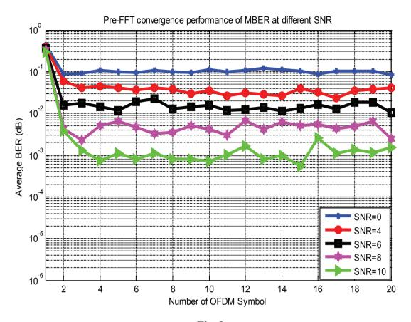
$\label{eq:Fig.9} \textbf{Pre-FFT beamformer Convergence performance at different SNR}$
