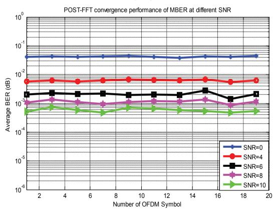
$Fig.\ 10$  Post-FFT beamformer Convergence performance at different SNR.
