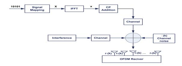
Fig. 1 The system model of OFDM transmitter
