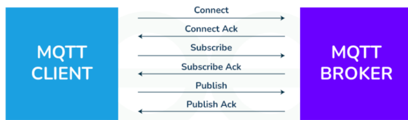
Figure 3.4: The message request-response in the MQTT protocol
