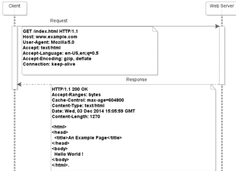
Figure 3.3: basic request-response model of communication between a web browser and a server over HTTP.
